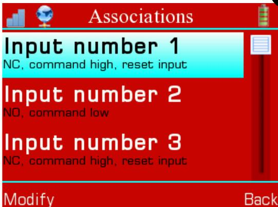
The **association menu** (Fig. 1) displays the trigger's list. These are formed by the names of the 6 triggers, by a trigger of "No line", by a trigger of "Low battery" and by a trigger of "Incoming call".
