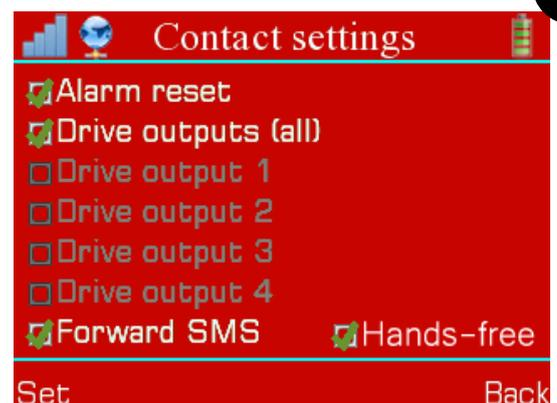
The **contact settings** are needed to give special remote control privileges to some contacts or to forward the DS 100 received messages to the corresponding number:
