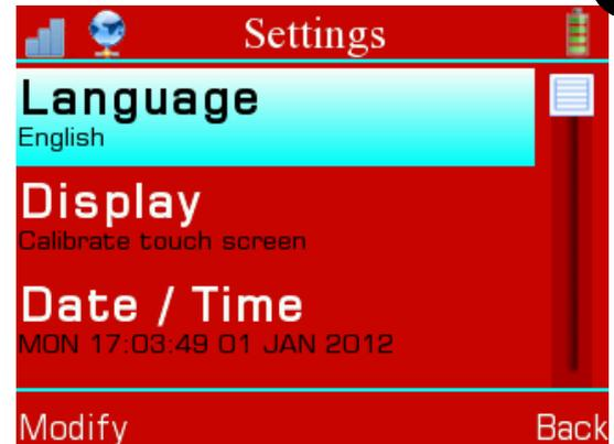
To **calibrate the touchscreen** we must select the “Display” voice in the settings list, and then press “Modify”. In the new screen press “Ok” to start the procedure, and then follow the instructions on screen.
