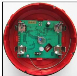
Picture 5 - inside view of the device: the PCB
