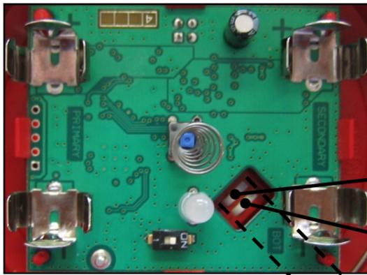
Picture 15 - the flash and light intensity selectors in detail
