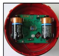
Picture 11 - primary and secondary batteries inserted
