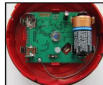
Picture 10 - secondary battery inserted
