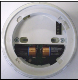
Picture 6 - primary and secondary batteries inserted
