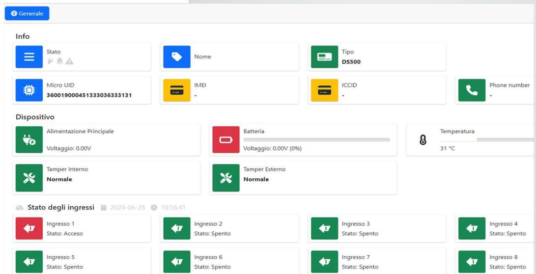
The screenshot shows a 'Generale' (General) tab for a device. It includes sections for 'Info' (Stato, Nome, Tipo DS500, Micro UID, IMEI, ICCID, Phone number), 'Dispositivo' (Alimentazione Principale, Batteria, Tamper Interno, Tamper Esterno), and 'Stato degli ingressi' (Input status for 8 ports).
